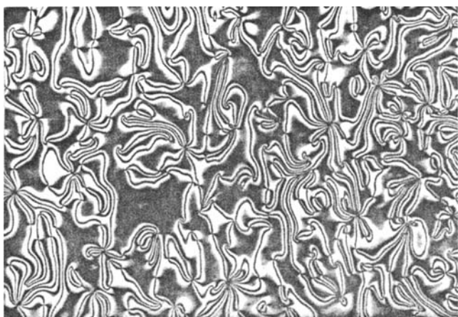
Figure 2. Polarizing microscope photograph of the schlieren texture of compound 4 at 449 K in the first cooling process.
